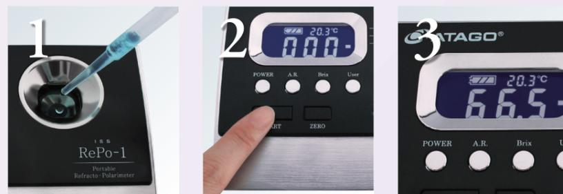
1 Fill the sample stage up to the fill line (approx. 3mL)
