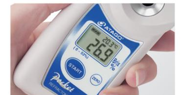
3 Measurement value and prism temperature are displayed in 3 seconds!
