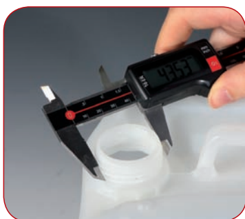
Measuring of canister thread
