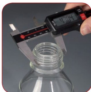
Measuring of bottle thread
