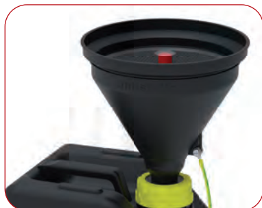
b.safe Funnels 180 with Level Indicator (Cat. No. R 840-16). Optic Level Indicator that is permanently mounted in the funnel. As soon as the red pin fills the inspection glass completely, the canister is full and has to be exchanged.
