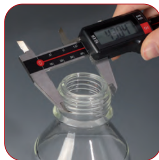
Measuring of bottle thread
