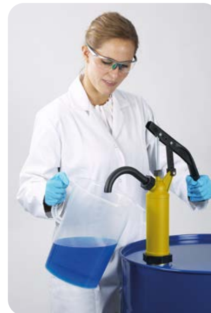
Lever pump with stainless steel piston rod The lever pump is made of polypropylene with a stainless steel piston rod made of AISI 304 (1.4301) and FKM seals.
