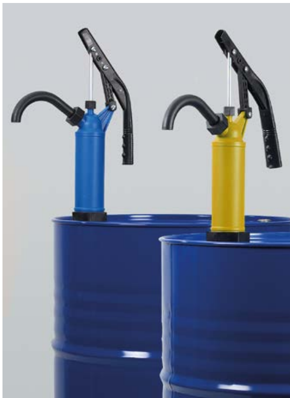
Lever pump with galvanised steel piston rod The lever pump is made of polypropylene with a galvanised steel piston rod and FKM seals.
