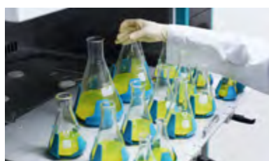
Rail-type platform allowing samples to be removed/mounted by pulling out the platform to the front.
