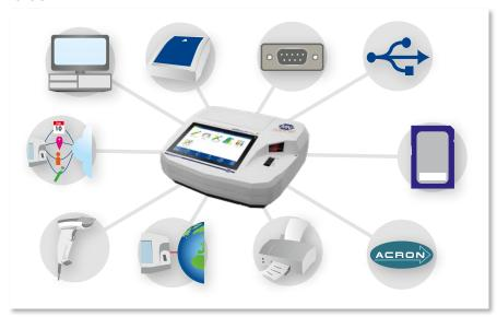
Easily accessible USB interface at the side of the instrument for the connection of a USB stick, printer or barcode reader.
