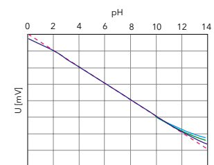
Exemplary mV curve of various electrode for different pH values. --- Ideal characteristic — Real characteristic for electrode 1 — Real characteristic for electrode 2 — Real characteristic for electrode 3
