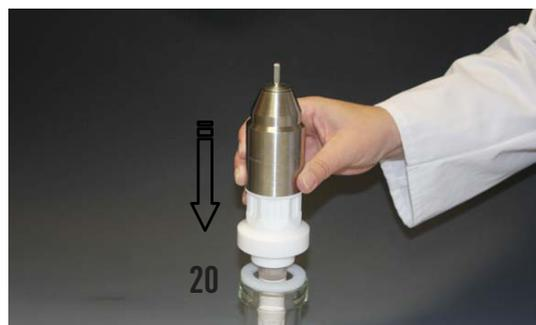
» Assemble the flange connection according to manufacturer's instructions. In case of temperature fluctuation, we recommend to use a flat flange with adjusting springs (without illustration).
