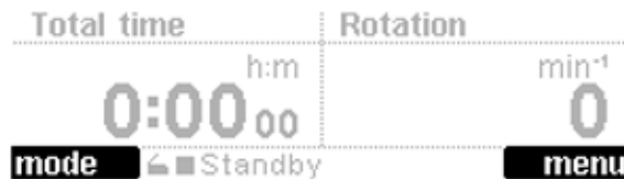
Fig. 17: Display of the assignment of the function keys; here: left key "mode", right key "menu"
