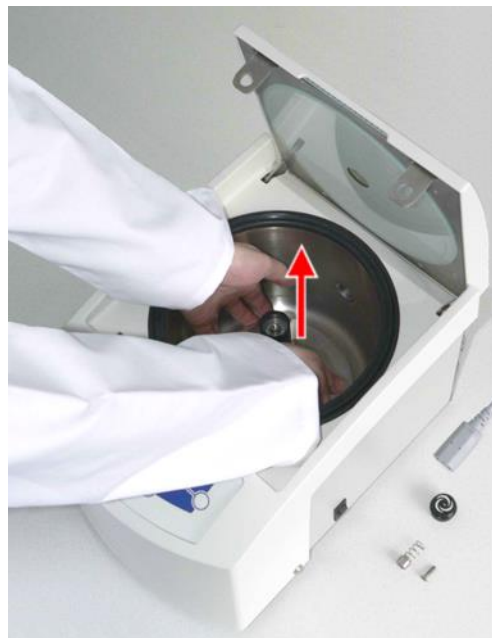
Fig. 44: Removing the rotor shaft
