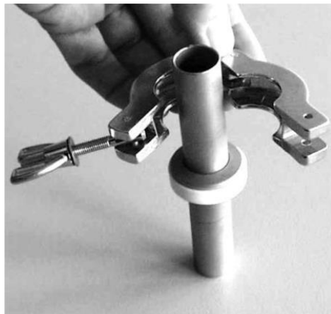
Fig. 40: Attaching the clamping ring
