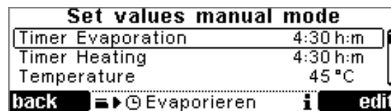
Fig. 27: Manual mode – selecting a set value
