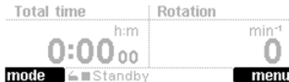
Fig. 21: Display of the assignment of the function keys; here: left key "mode", right key "menu"
