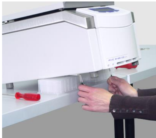
Fig. 50: Unlocking the lid locks
