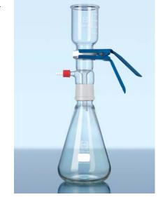
Furthermore, the filtering apparatus is suitable for the filtration of HPLC media, testing for bacterial contamination, residue analysis and the filtration of other media.
