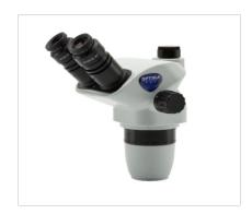
*Trinocular stereozoom microscope head,* 6.7*x*...45*x*
